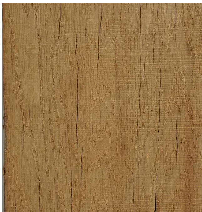
Figure 13-8. Surface checking on white oak 5/4 lumber.
