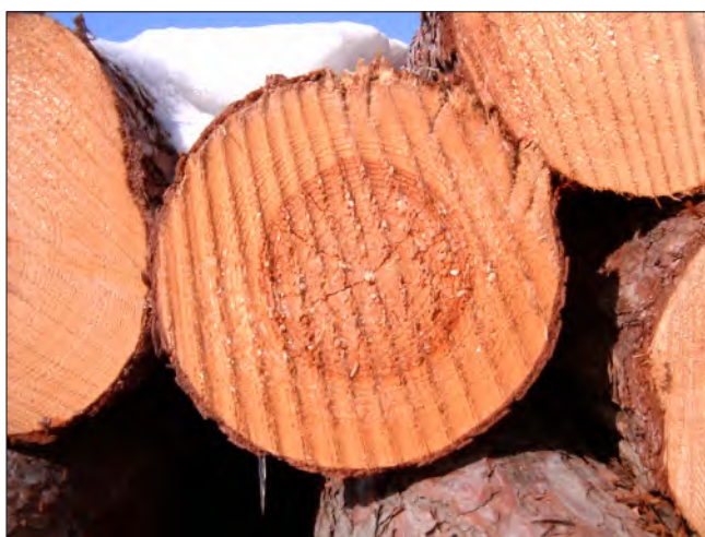
Figure 13-9. End checking in red pine logs.
